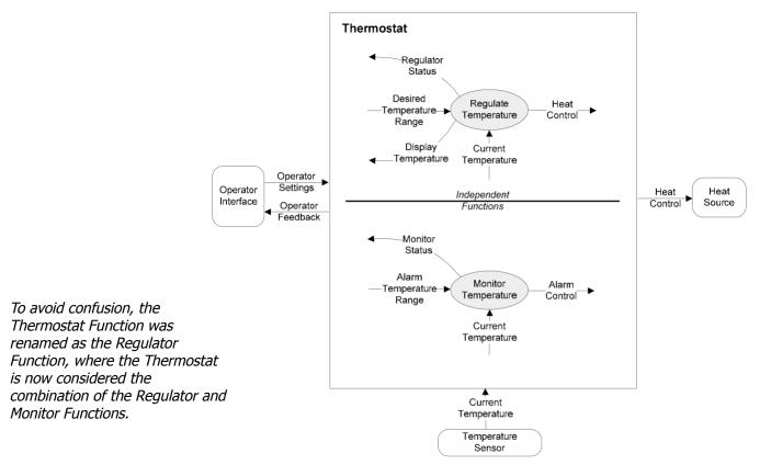
Figure 7. Revised Thermostat Dependency Diagram
