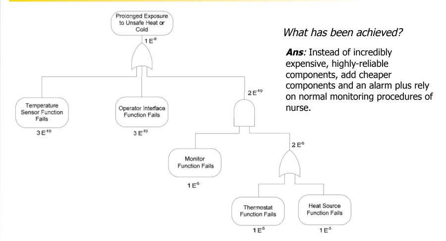
Figure 6. Revised Isolette Fault Tree
