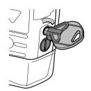
3. Insert the side the of key or the coin into the slot and turn clockwise until the latching button pops out. (The mark on the latch will line up with the open dot.)
